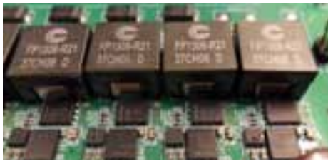
Example: High performance Server (PCB: 8 layer, 70 \mu\text{m} )
